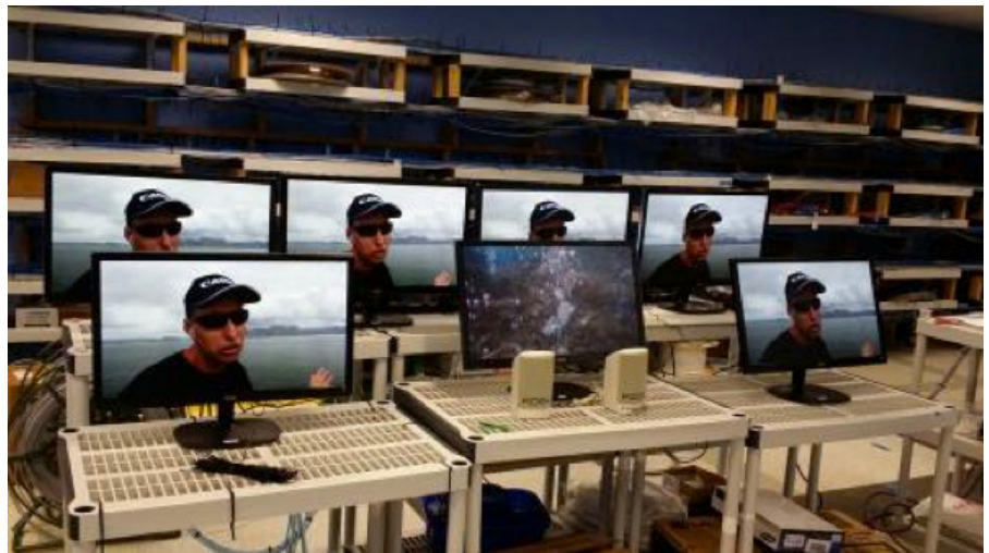
Figure 5. Display screens connected to HDBaseT receiver equipment showing clear pictures
